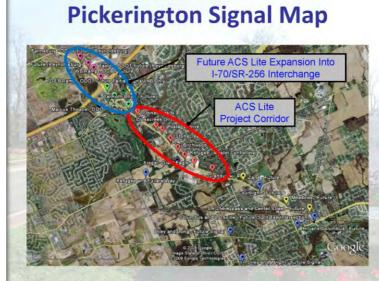
Pickerington's ACS Lite system cost \$338,000 (less than \$50,000 per signal). The system included upgrading and standardizing traffic controllers in the system, adding video camera detection at key intersections, installing ACS Light hardware and software and updating the signal communication with Ethernet over copper modems.
